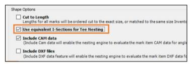
A new Tee nesting engine available in STRUMIS, will allow for nesting/optimization of Tee shapes and haunches out of standard beam profiles.
